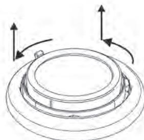
1. Hold the rotating housing on the activation hook, turn the glass retaining ring with glass to the left.
