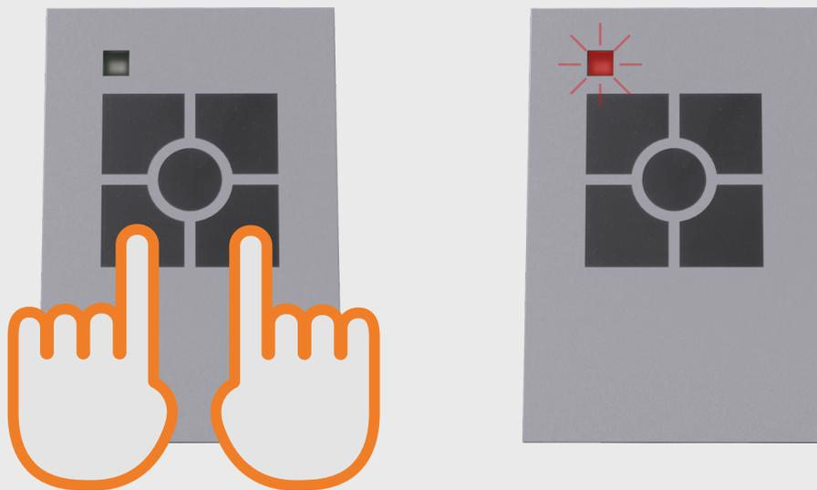
Now take the remote control and keep the two lower buttons pressed for around 10 seconds, until the upper left LED starts to flash in red. You should proceed the step on the following page within 10 seconds after you have released the Buttons.
